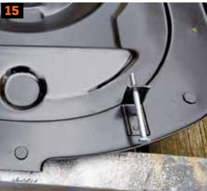
**15.** Smallblock setups have tabs welded to the bottom of the retainer. These accept the braces shown in Photos E and J in the parts section.
