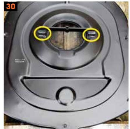
30. The finished product. On this car, we needed to raise the carb strap-bar about one inch, too (circled). You can weld, right?
