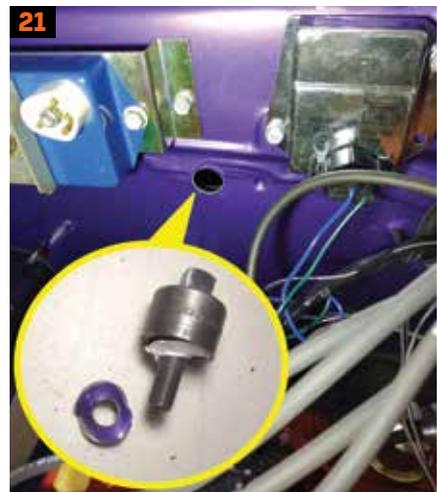
**21.** Use a Greenlee punch, 1/4" diameter, backed up with cardboard (to not mar the paint), for the control cable grommet. Brush some primer on the bare steel.
