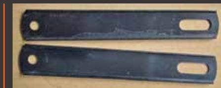
**E)** ...the 340 uses brackets (s) which attach to the front of each cylinder head. You'll see more of this as we perform the installation.
