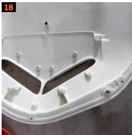
**18.** Feed the intermediate cable through the slot in the rear (on the pass. side) of the retainer, then...
