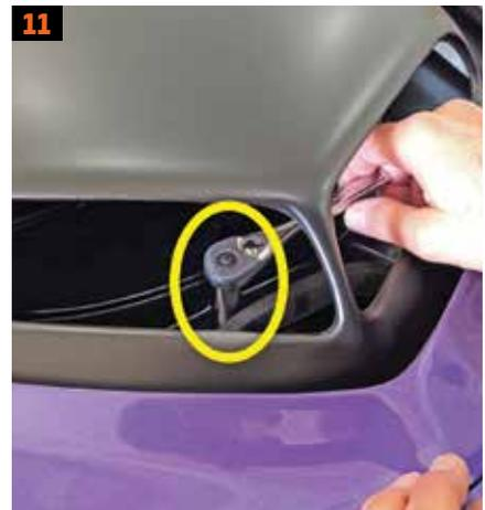
11. Next, tighten the fasteners—as many as you can reach—through the grille openings. Open the hood and tighten the remainder.
