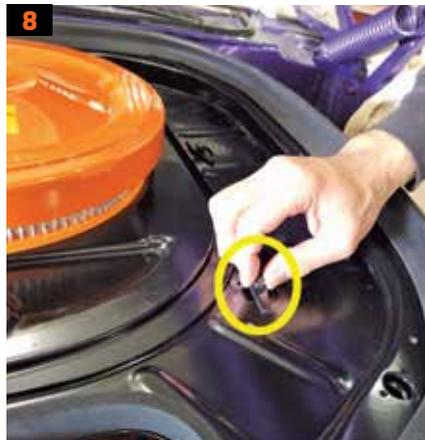
8. Install the retainer and adapter, using the oddball diamond washers, make the nuts just snug. Also install the air cleaner.
