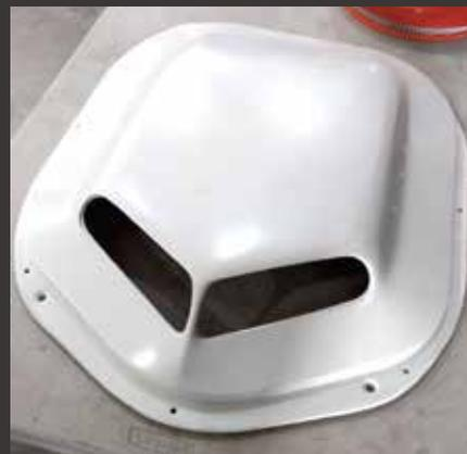
**F)** The Shaker bubble, as supplied by Tommy, is very nearly ready for paint, with a smooth gelcoat surface finish.
