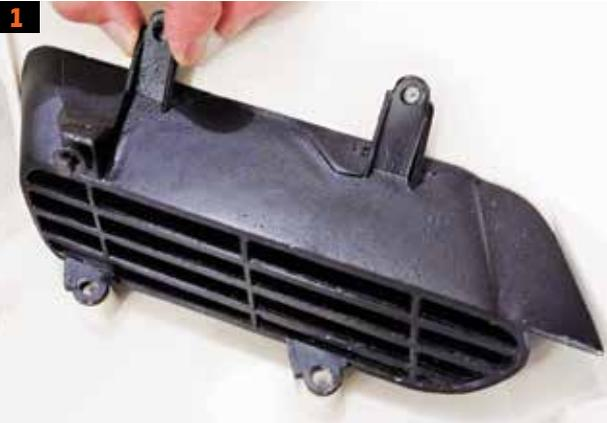
**1.** Begin the installation by trial-fitting the grilles (shown) and air doors. Make the locations that will need to be drilled.
