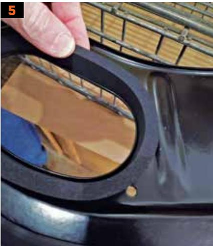
5. Also apply the seal to the hot-air opening.
