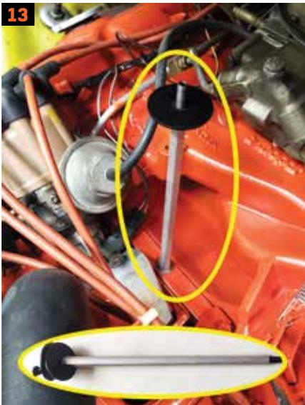
**13.** If you have a B-engine (383), remove the center screw from the intake manifold gasket front reinforcement and replace it with the long hex stud and the short double-ended stud.
