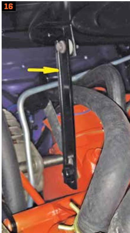
**16.** The smallblock braces screw to existing holes in the cylinder heads' front surface. 440 4-Bbls use shorter brackets, Plastisol-coated (see Photo D above) which simply rest on the valve covers. Multi-carb engines have no brackets, none are needed.
