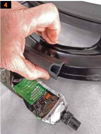
4. Using weatherstrip contact cement, install the perimeter seal. The factor joined the ends on the right side, we chose the rear (less visible). Join the ends using the supplied tape seen in Photo J above.
